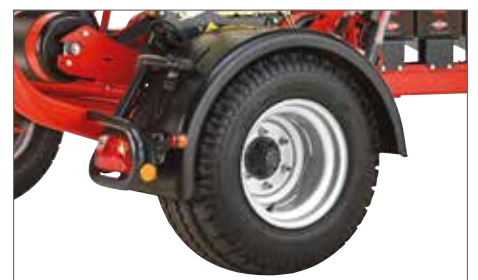
Large mudguards will prevent the film being damaged during transport
