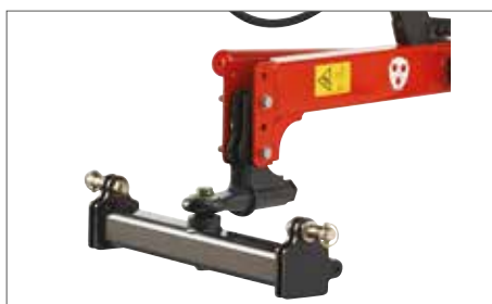
The long drawbar makes it easy to tow the wrapper sideways with wide / larger tractors
