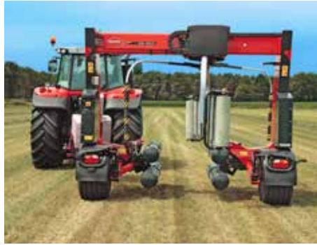
The wrapper folds from its 2,5 m transport position into 4 m wide field position
