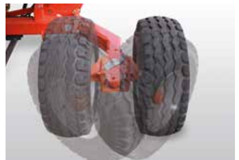
Limited transport width due to adjustable wheel positions
