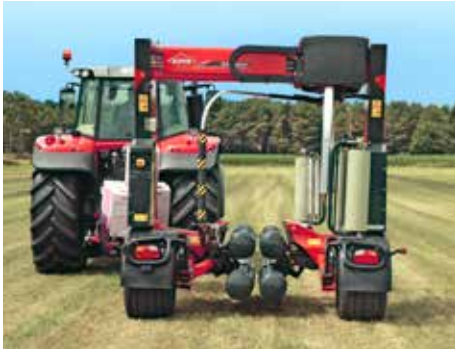
The wrapper folds from its 2,5 m transport position into 4 m wide field position
