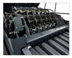
4. Double knotting system with standard electronic monitoring
