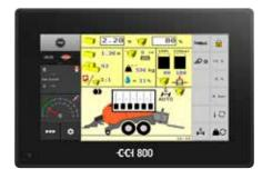
**CCI 800: The compact ISOBUS terminal** The 8"/20.3 cm screen displays the main machine and miniviews on the side. Click on one of the mini-views to switch it to the main screen.
