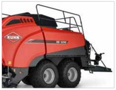
**Everything for your safety** For more safety, the knotter deck is equipped with solid stairs and a safety railing.The safety railing can be folded down easily to reduce the height of the machine during transport.
