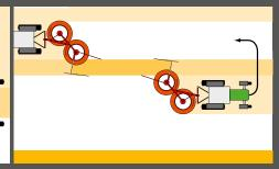
Double swath raking, working width 600 cm (19'8")
