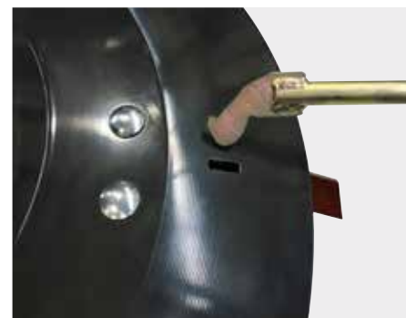
4. Knife changing system with special tool and knife holder
