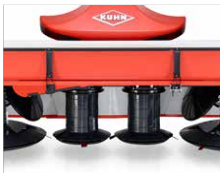
5. Standard swath discs securing a narrow swath
