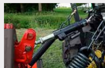
FRONTFLEX telescope top link (only in combination with a fixed headstock)
