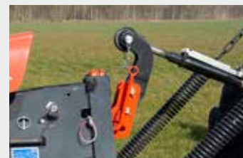
FLEXTOP flexible top link connection (only in combination with a fixed headstock)
