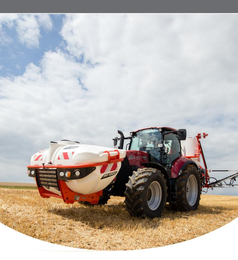
Front-end sprayers are not simply front tanks; their design is based on boom sprayers and makes them autonomous and independent. PF combined with Deltis or Altis 2 rear sprayer increase autonomy up to 100%. It is also predisposed to be combined with an autonomous fertilization or spraying kit for a localized application on a rear implement.
