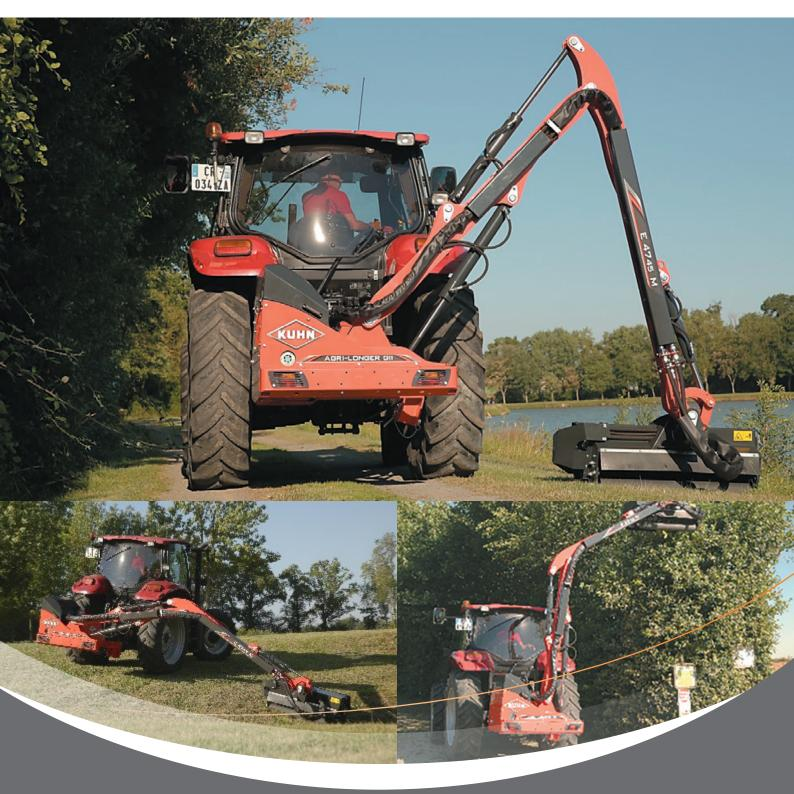
The AGRI-LONGER GII 4245 M and 4745 M have the same design, hydraulics and arm of the AGRI-LONGER GII 5045 P. However, like the AGRI-LONGER GI, they have a pendulum link system for mechanical safety.
