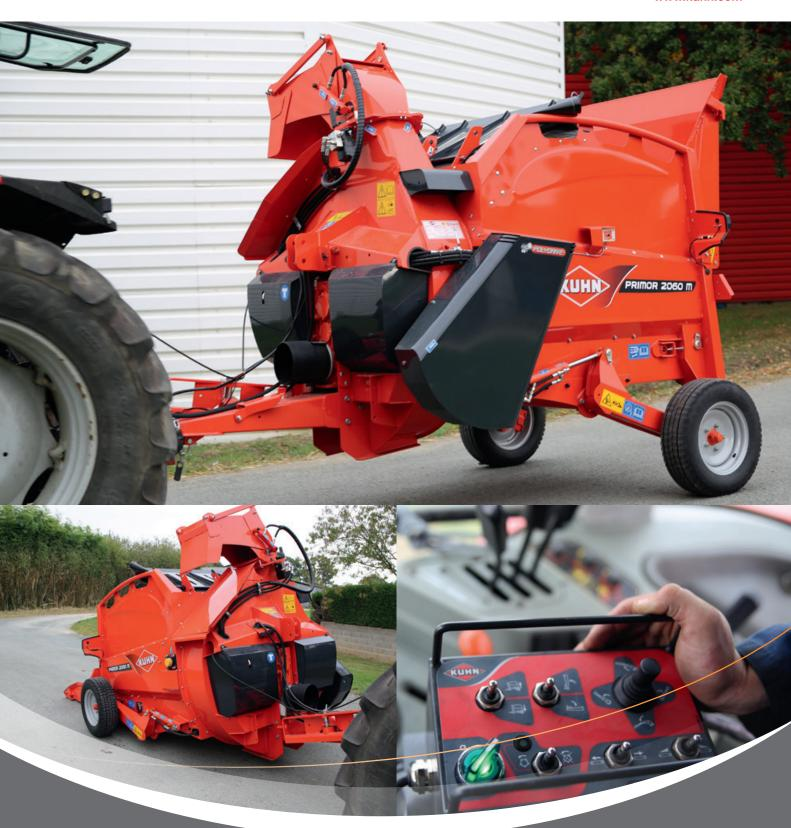
The PRIMOR 2060 M semi-mounted version is an additional model to the straw blower and all-fodder feeder range with a **new model adapted for low-power tractors requiring fodder distribution**. This machine allows to load either one rectangular bale (up to  $1.30 \text{ m} \times 1.20 \text{ m} \times 2.70 \text{ m}$ ), or 1 round bale (up to 1.80 m in diameter) independently with an adjustable axle mounted on two cylinders.
