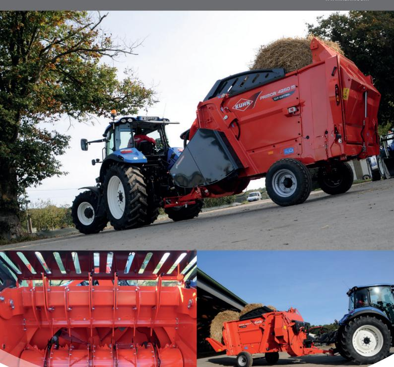
The PRIMOR 4260 M CUT CONTROL brings an additional feature to the straw blower and all-fodder feeder range: the **possibility of activating (or disabling) the chopping function**. The same machine can therefore be used to **put down short straw (cubicles) or long straw (bedded packs)** while retaining the capacity to deliver long-fibre fodder (such as hay or haylage).
