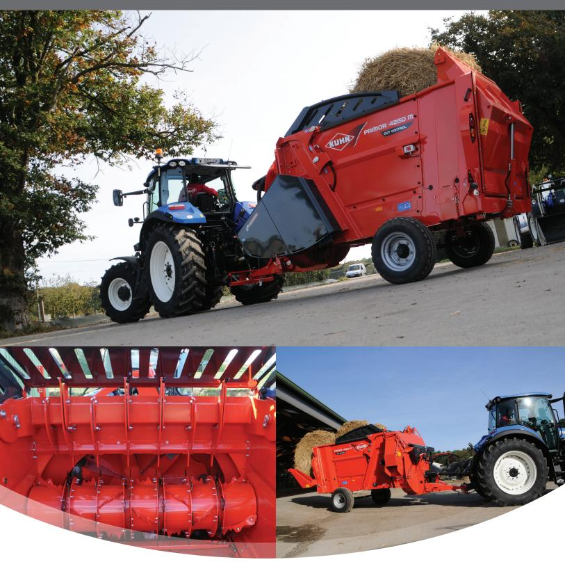
The PRIMOR 4260 M CUT CONTROL brings an additional feature to the straw blower and all-fodder feeder range: the **possibility of activating (or disabling) the chopping function**. The same machine can therefore be used to **put down short straw (cubicles) or long straw (bedded packs)** while retaining the capacity to deliver long-fibre fodder (such as hay or haylage).
