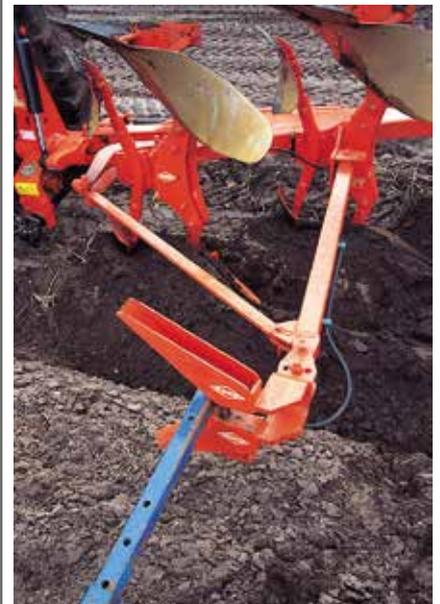
Available for the complete plough range the arm allows the use of a furrow press with easy hooking up and hydraulic push-off. On the pick-up hook part of the arm where there is most risk of damage all grease nipples and hydraulic hoses are protected inside the structure of the head. The arm folds up conveniently for subsequent transport.
