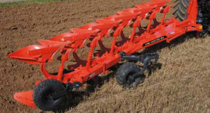
The wheel is equipped with a central pivot allowing it to automatically follow any changes in working width. The depth is adjusted by turnscrew **1** (or hydraulically **2** with the possibility to adjust the depth differently on each side. The depth wheel can be mounted in many different positions along the beam in order to achieve the best possible configuration.
