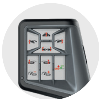
9-function divider of the mower conditioner with conveyor
