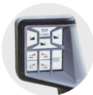
9-function divider of an ISOBUS AXIS fertilizer spreader
