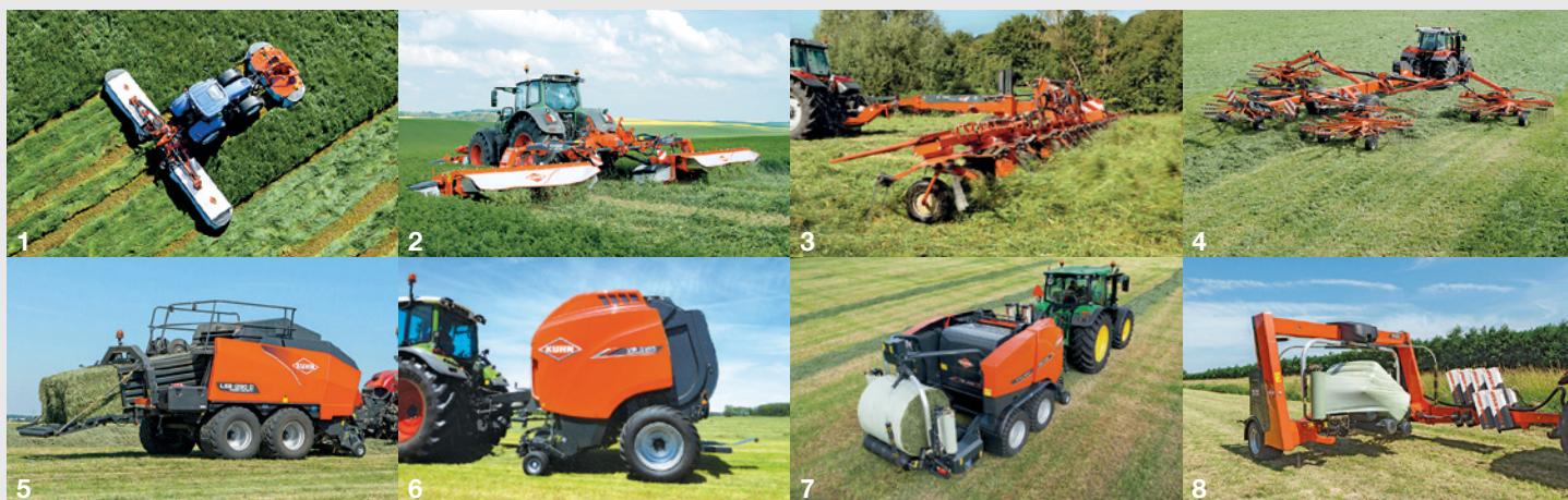
1. Triple gang mower - 2. Triple gang mower conditioner - 3. Large-width tedder - 4. 4-rotor rake - 5. High-density baler - 6. Round baler - 7. Fixed-chamber baler-wrapper combination - 8. Wrapper.
