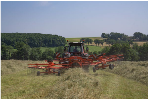
Caption: The rotors can be lifted individually during work to avoid moving grass multiple times
