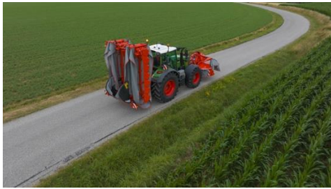
Caption: The GMD 15030 has a transport width under 3m and a folded height of under 4m, which is similar to KUHN's other triple mowers
