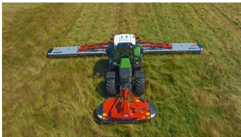
Caption: KUHN's GMD 15030 features four 3.1m, seven-disc beds and can operate at 14.5m wide when used with a 3.1m GMD front mounted mower
